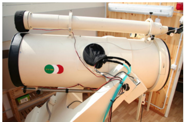
Figure 1– The author's 600 kg Schmidt telescope
